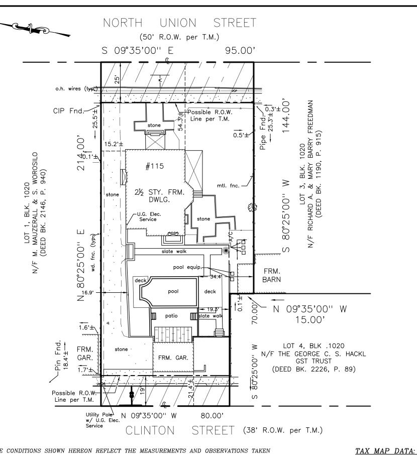
1.) THE CONDITIONS SHOWN HEREON REFLECT THE MEASUREMENTS AND OBSERVATIONS TAKEN FROM FIELDWORK PERFORMED ON DECEMBER 19, 2018.
