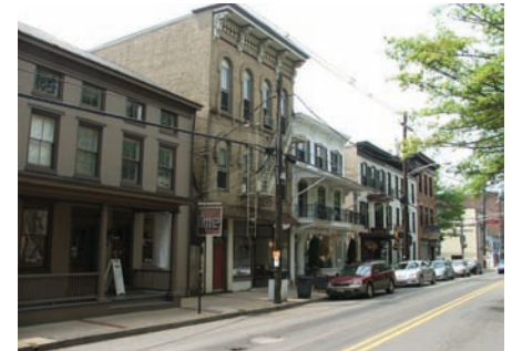
This block of buildings was constructed over two decades, but the pattern and orientation of window openings and the overall ratio of wall to windows (solid to voids) is very similar. This gives the block visual continuity.
